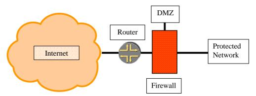
Figure 1: Internet-router-firewall-protected network setup
