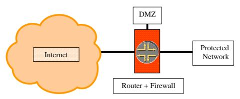
Figure 3: Internet-Edge-protected network setup
