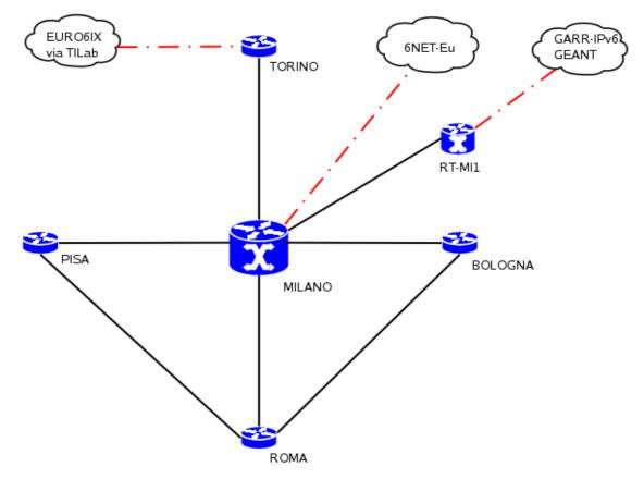
Figure 5: The 6NET topology in Italy, as of September 2004.
