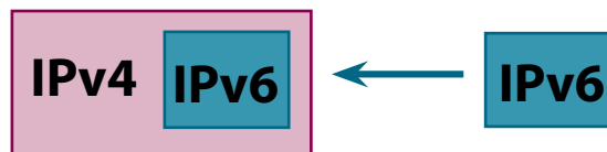
FIGURE 6: IPv6 ENCAPSULATED IN IPv4
