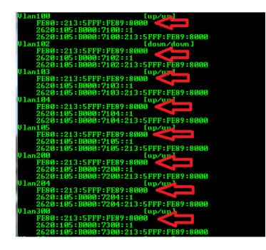
Figure 1 - All SVIs have the same link local address because they use the same virtual MAC address for their interfaces.
